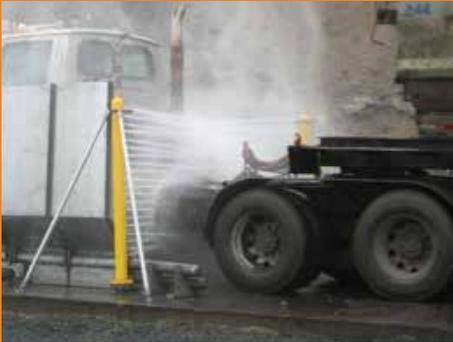
The high impact side spray towers offer effective cleaning into wheel wells and lower detail of the vehicles.
