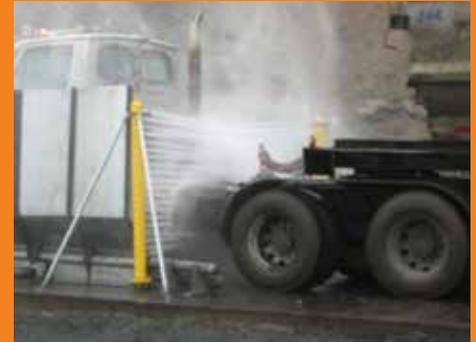
Our tire wash platforms can be installed to accommodate wider than street legal vehicles such as articulated dumpers or haul trucks. The wash elements are of high quality galvanized steel construction. The package can be upgraded to SS 316 or SS 304.
